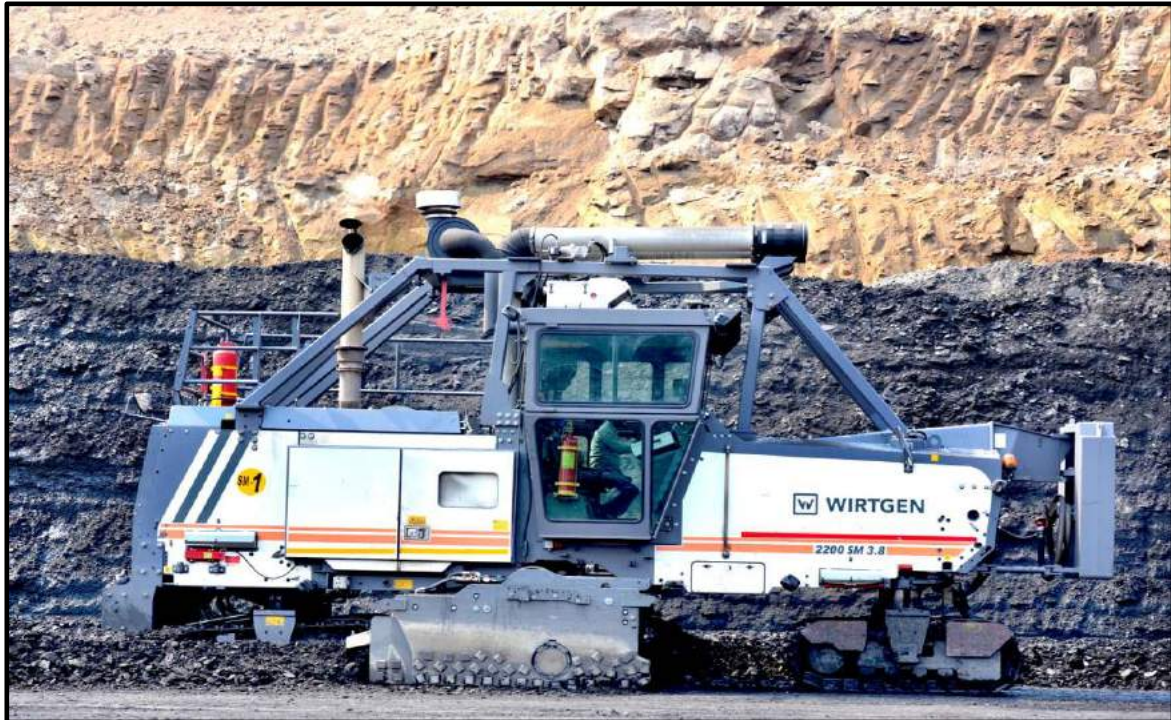
Surface Miner at Penganga OC along with dust suppression system
