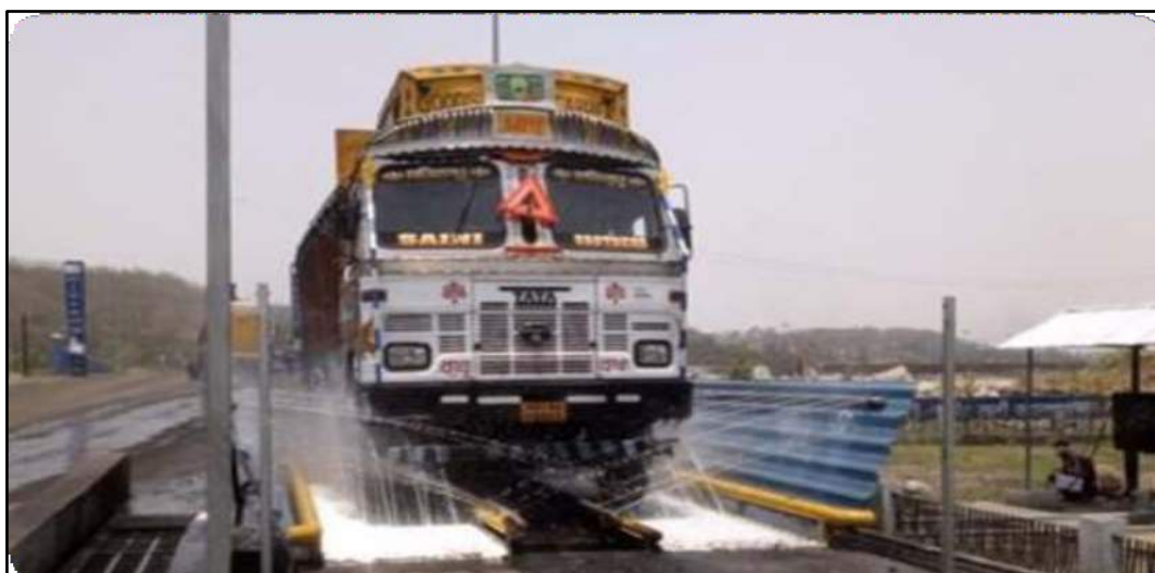
Automatic tire washing system, Umrer OC
