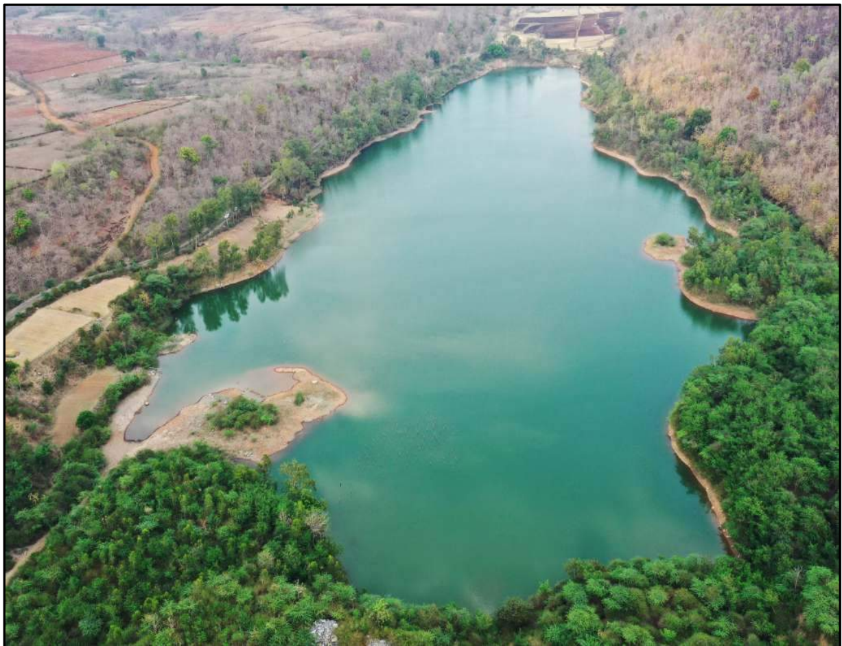
Augmentation of Ground water recharge-Mansarovar, Mine void of New Sethia OC in an area of 17.50 ha holding 12 Million Gallons of mine water
